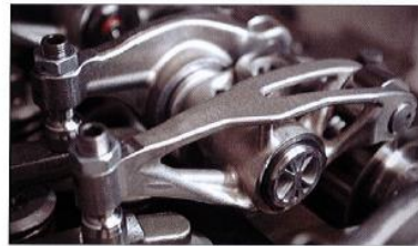
The re-designed metal AM version of the rocker arm is shown during a bench test inside a Euro 6 engine
