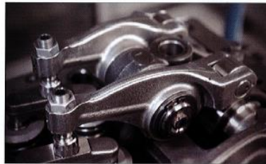
The original rocker arm in a Renault Trucks Euro 6 DTI 5 engine
